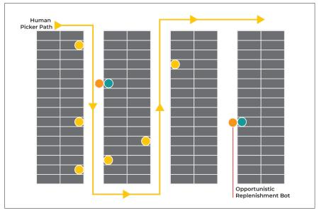
Picker encounters a replenishment bot along the pick path and executes the replenishment. The second replenishment bot is not along the pick path, and therefore, would be served by another pick cycle.
