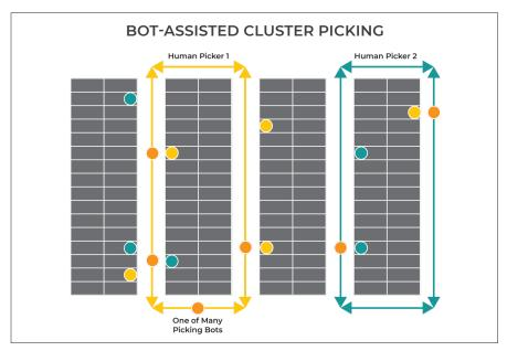
Illustration has bots traversing the pick paths, waiting for a picker to execute the pick. Meanwhile, a picker walks along a designated pick area looking for bots requesting a pick, executes the pick and moves on to the next request/bot. It's possible for a picker to walk the designated area multiple times to execute all of the picks, which might decrease the savings implied by the illustration.
