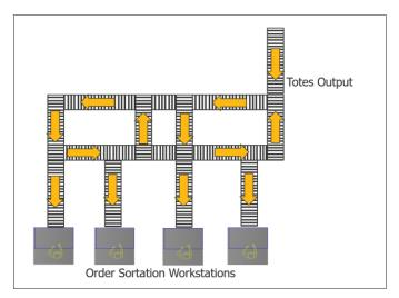
Illustration (left): shows a traditional solution for transporting totes into a set of stations using conveyor segments and loops to allow recirculation and crossovers.
