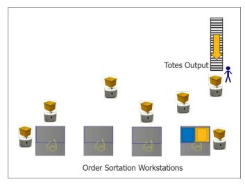
Illustration (right): demonstrates the lower cost bot sorter in which the bots move the totes between the input/output location and the workstations.
